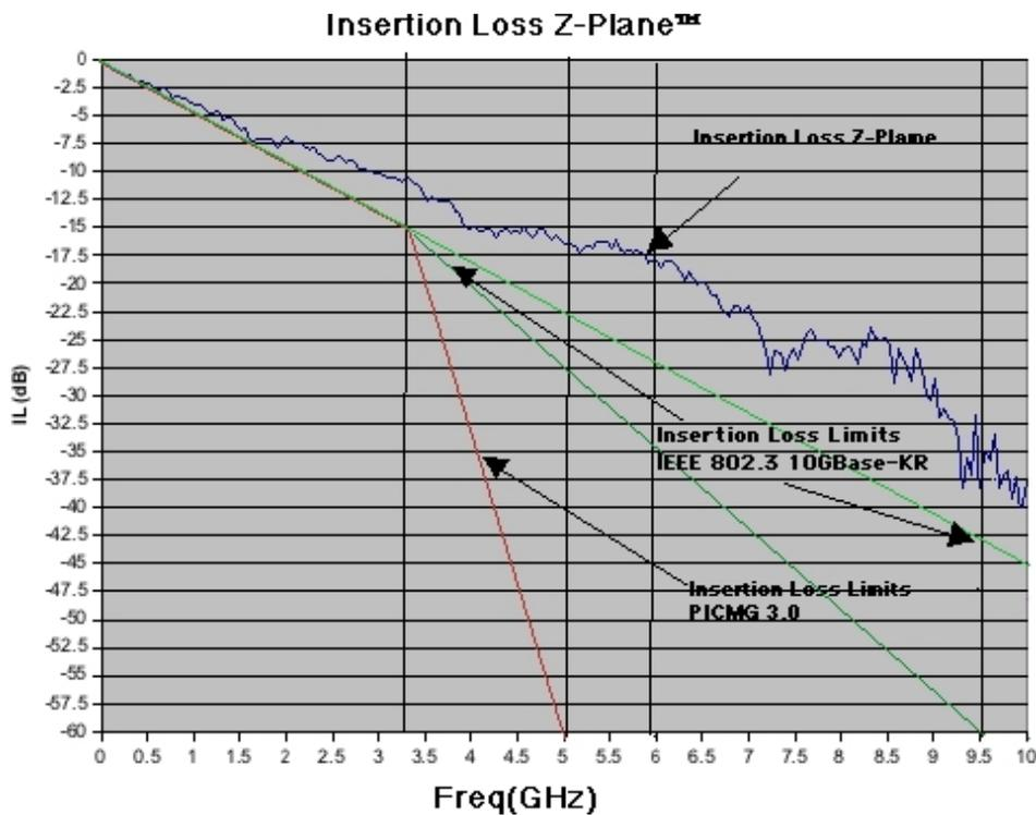
The thick board (0.134") has standard lower impedance terminations to the backplane, but is otherwise well matched, and this too will meet or exceed the requirements.
